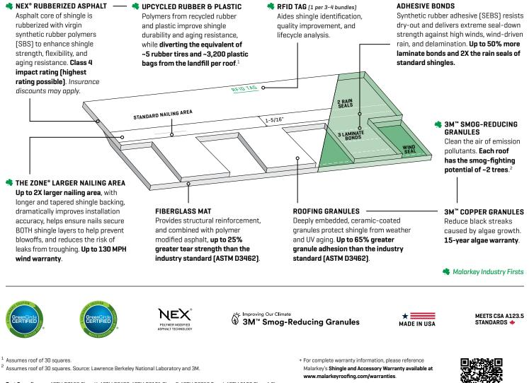
Test Compliance – ASTM D7158 Class H, ASTM D3462, ASTM D3161 Class F, ASTM D3018 Type I, ASTM E108 Class A Fire Rating, UL 2218 Class 4, CSA A123.5, ICC Approval – ESR-3150, ICC-ES AC438, and FBC Approval – #14809.
