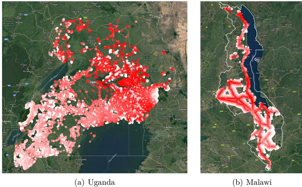
**Figure 2.10:** Suitability of locations to on-grid solar PV
