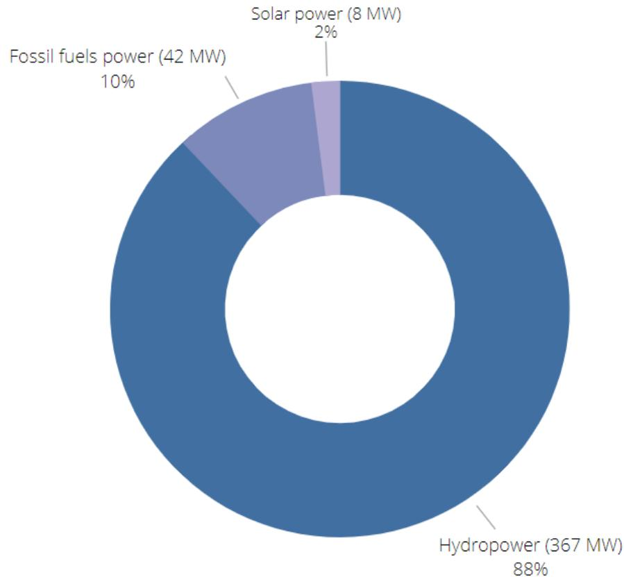
**Figure 1.9:** Malawian mix for electricity production in 2019
