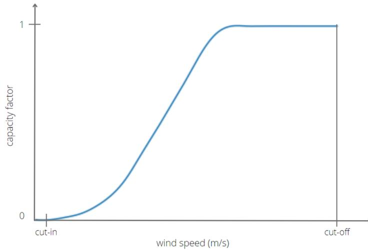
**Figure 2.2:** Power curve of a generic wind turbine
